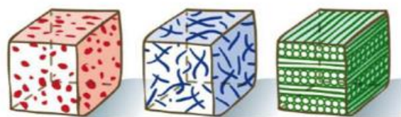
Fig. 1. Composite material types, from left to right: dispersed, fiber-reinforced, stratified
